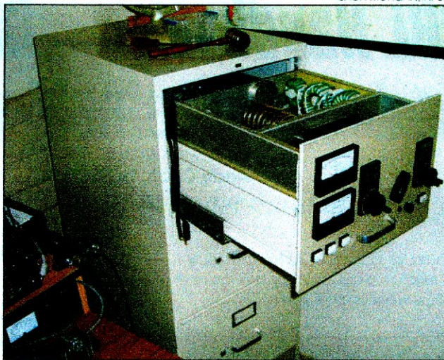
Figure 3 — The amplifier mounted in a drawer of the legal "amplifier" cabinet.
