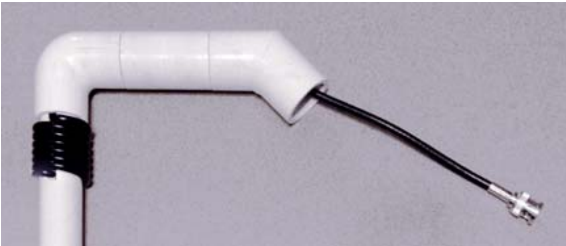
Figure 2: Handle of the walking stick showing the 7-turn choke and the feedline pigtail. You may mount a connector instead, if you prefer.
