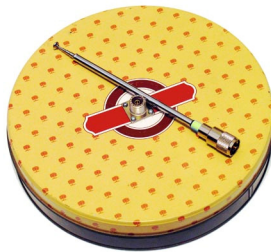
Figure 7: 10 in. cookie can with telescopic whip in a UHF connector. Whip and coax are put inside the can for storage.
