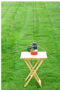
Figure 9: Coffee Can Antenna with 19 in. spike and 4 drooping 21 in. radials
