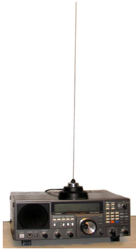
Figure 8: A magnetic mount and spike placed directly on top of a rig.
