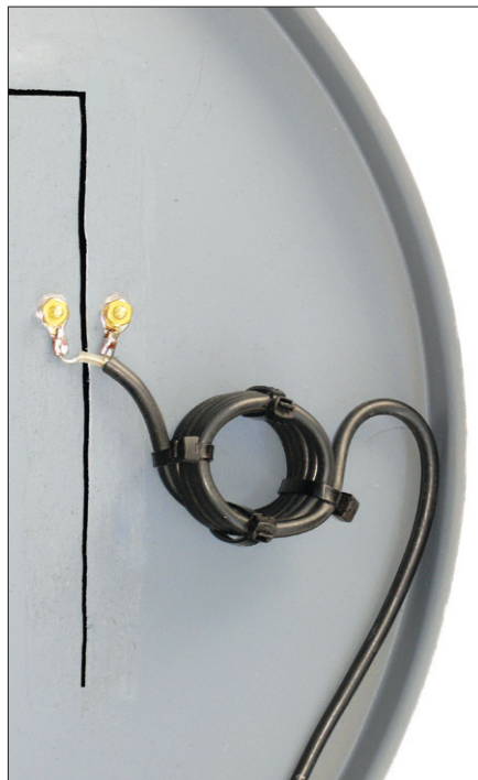
Figure 6 — The coax feed line includes a six-turn coiled-coax choke balun and attaches 4.5 inches from the slot end.
