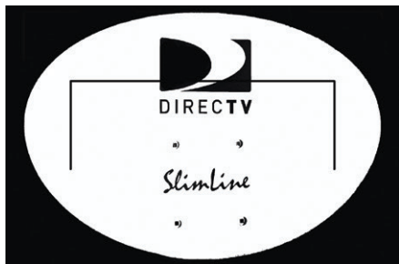
Figure 4 — A horizontal slot antenna, with drooping ends, cut into the reflector of a Slim-Line DIRECTV satellite dish.
