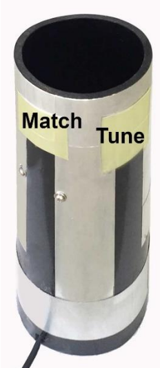
Figure 2: Vent antenna before painting. Note highlighted shorting tapes.
