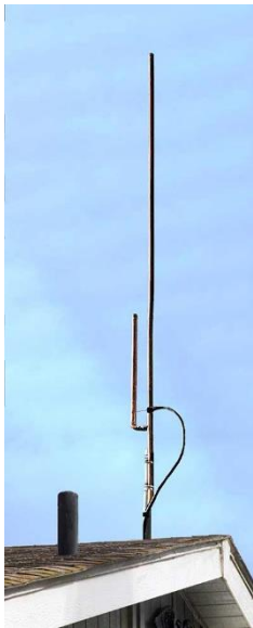
Figure 1: My home-brew J-pole next to the vent-pipe roof-topper.
