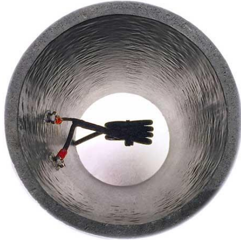
Figure 5: Internal feed point and coax balun
