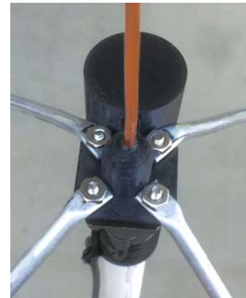
Figure 4 — Radials fashioned from 1/4-inch metal tubing and attached to the fixture with 6-32 hardware.
