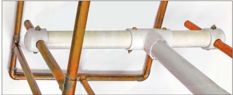
Figure 6 — Mounting assembly. Note \frac{5}{8} -inch holes through the end caps and 10-24 x 2 inch screws.
