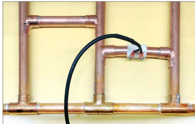
Figure 5 — Movable bars, tune (left), and match (right). Also, note the feed point.
