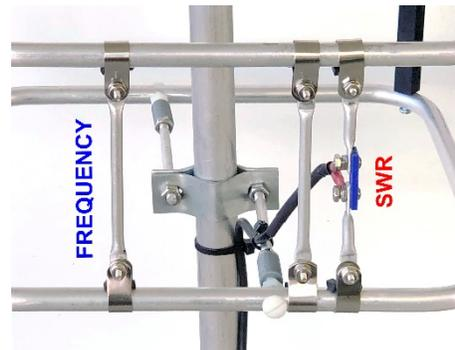
Figure 3: Vertical interconnect sections, Left: Frequency adjustment. Right: SWR adjustment (feedpoint).
