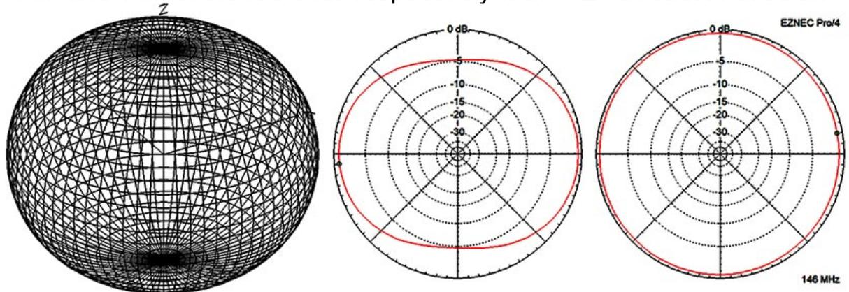
Figure 5: Left to right: Free-space 3D radiation pattern, elevation (vertical) pattern and azimuth (horizontal) pattern. Gains in dBi.
