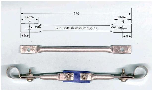
Figure 7: Vertical interconnect sections. Lower section with clamps.. Note plastic insulator in the feedpoint section (lower).
