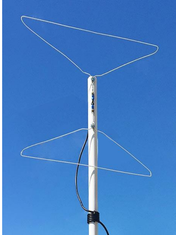
Figure 1: Our archetypal ultra-simple home-brew ham project, a coat hanger 2m base-station vertical
