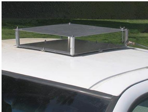
Figure 1: Antenna on cab of pickup truck, attached by neodymium cup magnet mounts
