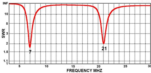
Figure 5: SWR curve. 40 meter dipole
