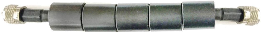
Figure 4: 1:1 ferrite sleeve current choke balun
