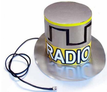
Figure 1: Lincoln-style aluminum stovepipe hat antenna
