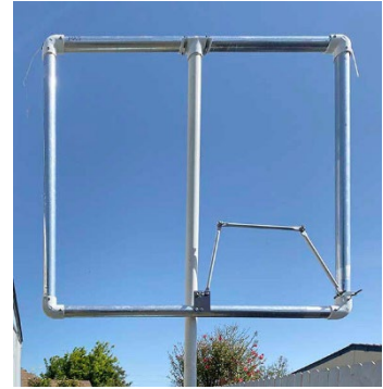
Figure 1: A low-cost 45-inch square optimized foil tape and PVC magnetic loop example
