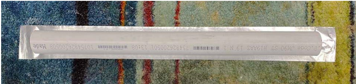
Figure 10: Applying foil tape to the 42 in. 1½ in. PVC pipes (four)
