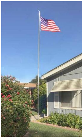
Figure 5: My stealthy 20 ft. HF HF flagpole fed with foam-encased open-wire line lying right on the ground
