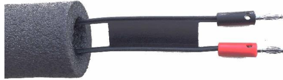
Figure 2: 450 Ohm window line encased in the polyethylene foam tubing for insulating \frac{3}{4} in. pipe
