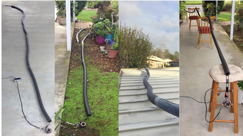
Figure 1: Adverse, non-open-air, situations for 450 Ohm window line: (1) on dry concrete, (2) lying on wet garden soil (3) directly on an aluminum patio roof, (4) in the open (comparison reference)
