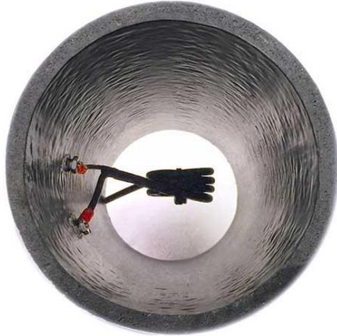
*Figure 5: Internal feed point and coax balun*
