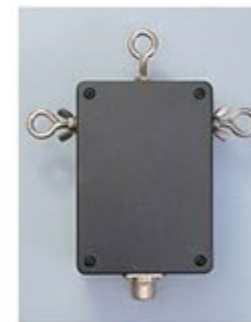
The finished balun in a small plastic box, with eye bolts on the sides for attaching antenna wire and a bolt on the top for suspending the balun.
