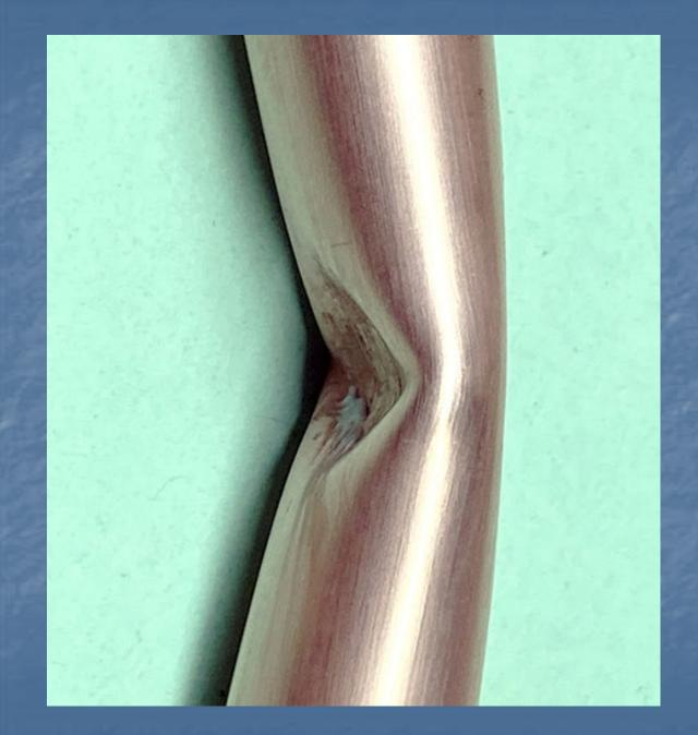
10 ft. lengths **Partially flattened** and bent at 2 ft. to be parallel at the bottom
