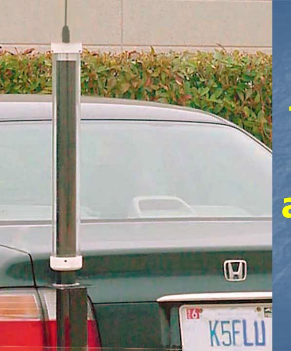
Just a Plain Coil to add inductance to make a short antenna work on a lower frequency
