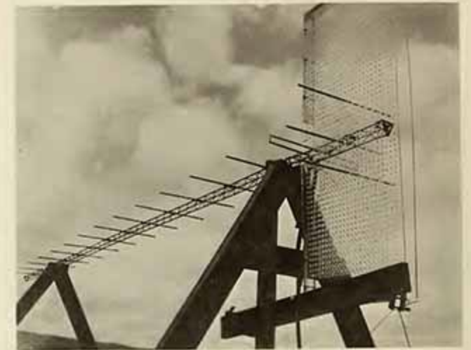
FIG. 3 - PHOTOGRAPH OF THE TRIGONAL REFLECTOR EXPERIMENTAL SET-UP USED WITH THE 4.2λ YAGI
