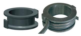
Figure 8: 3D printed quick-form for a VHF balun using RG-58 or Mini-8 coax.
