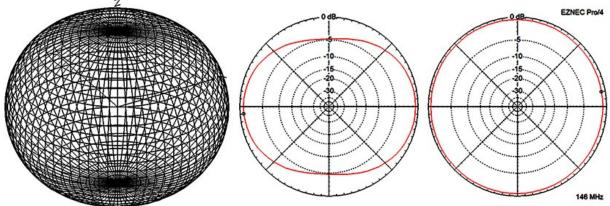
Figure 5: Left to right: Free-space 3D radiation pattern, elevation (vertical) pattern and azimuth (horizontal) pattern. Gains in dBi.
