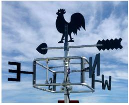
Figure 1: Concealed 2m antenna. The Rooster-Tenna
