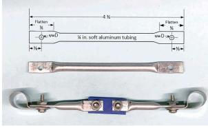
Figure 7: Vertical interconnect sections. Lower section with clamps.. Note plastic insulator in the feedpoint
