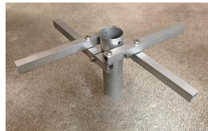
Figure 11-10: Hand fabricated mast top assembly from ¾ in. square aluminum tubing and bolts.
