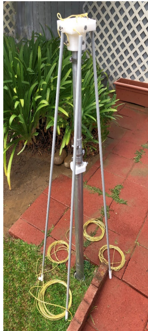
Figure 11-7: Mast and spreaders collapsed. Notice PVC conduit ground support pipe, top just visible. Auto-tuner not shown.
