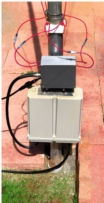
Figure 11-7: LDG RT-600 remote auto-tuner and remote directivity switch box. Balun just out of view.
